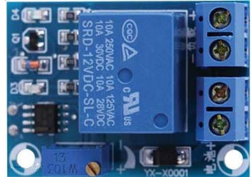
**NOTE: Minus (-) Battery & Load are Internally Connected**
